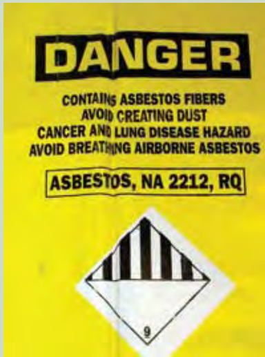
Example of asbestos-containing waste labeling
