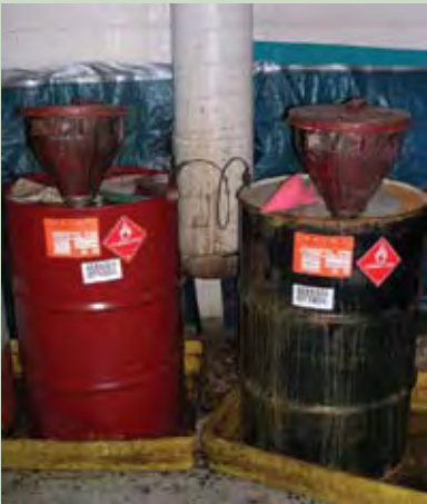
Bonding and grounding of flammable liquids containers
