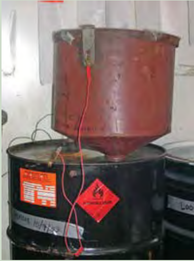
Bonding and grounding of flammable liquids containers
